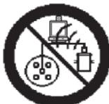
Install far from the ignition coil and pass the wiring far from the high voltage cables.
